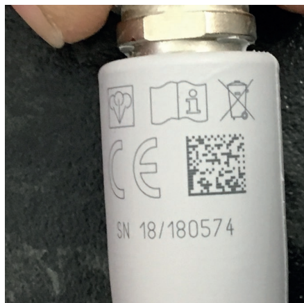
Figure 4: Essential regulatory graphics and a unique ID matrix code on a medical cord set
